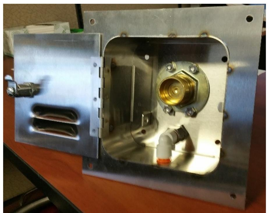
Chart's Parker 540 P style fill line and Series N style nylon vent line have been replaced by Accuflex 3768 series liquid CO2 fill line and Accuflex 1416C series CO2 vent line. The Accuflex series fill and vent lines have been selected for use in Chart Bulk CO2 Beverage systems because of their compatibility with beverage grade CO2, and they have been tested for exposure to temperatures down to -109.4°F by utilizing a flexible bend test. Key specs on the fill and vent lines are:
