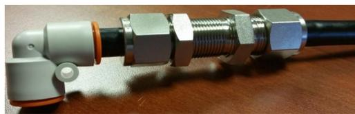
The Accuflex 1416C vent line must use compression fittings and should not be used with bar style fittings. The fill box depth dimension has changed to three inches deep to accommodate these new bulkhead compression fittings. The liquid CO2 fill connection has not changed on the new design fill box. It will accommodate all fill lines that have 45 degree flare fittings.
