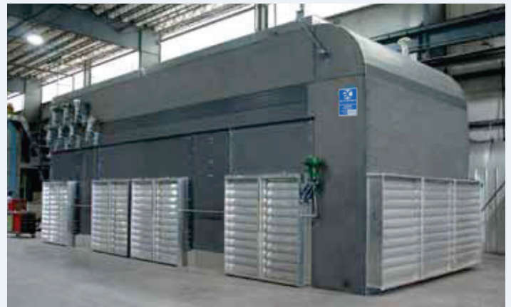
Optional over-the-end warm air recirculation system
