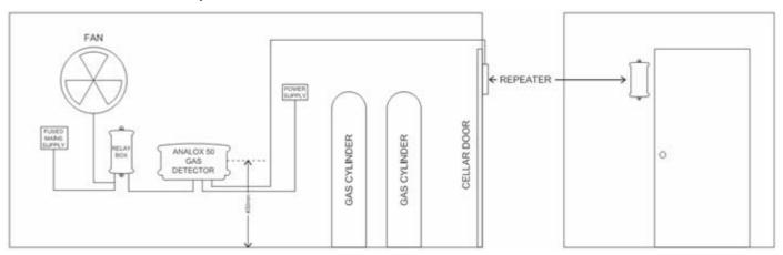
Attach the main unit to the wall 450mm from the floor as close to the valves and manifolds as possible. An 8 metre 8 core cable is pre-wired to the Ax 50<sup>TM</sup> and has a Remote Alarm Repeater pre-attached. Run the Remote Alarm Repeater cable to the outlet door, safely securing the cable with cable clips.
