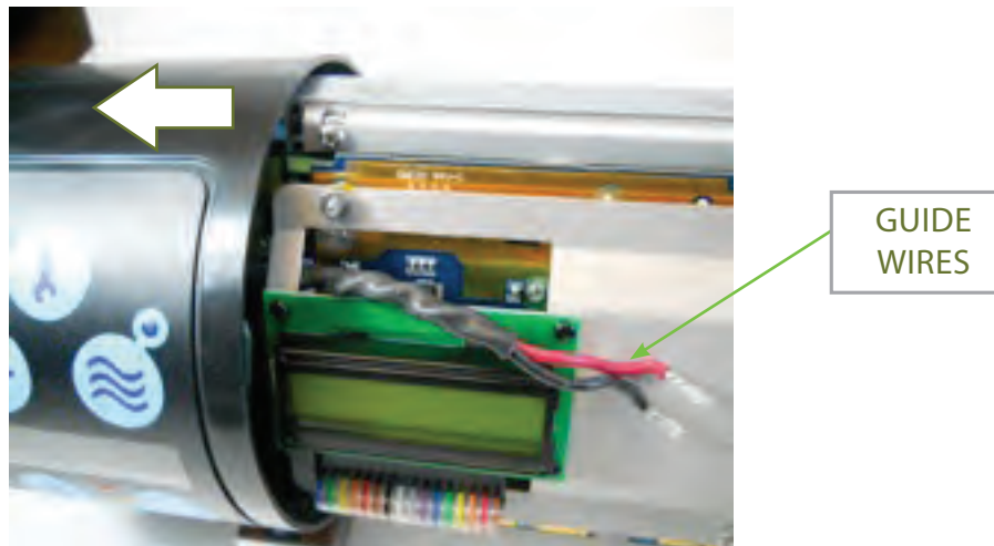
Figure 26: Inlet Cap Removal
