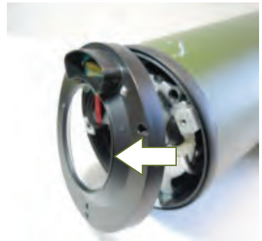
Figure 15: Removal of the 3 Rain Guard Screws
