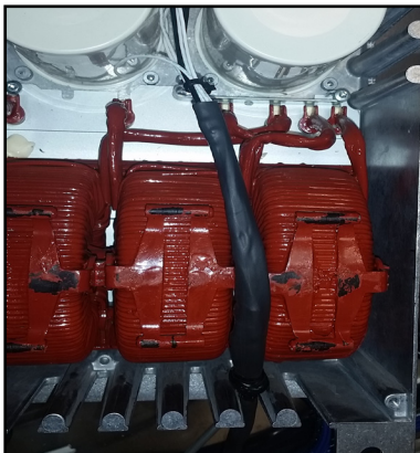
Figure 11 - Wiring Routing in VFD.
