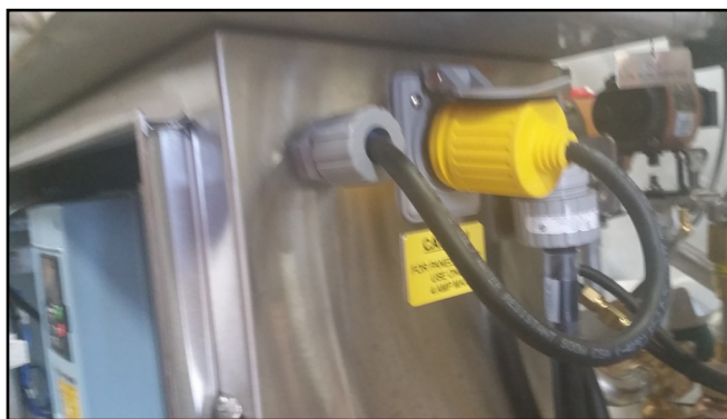
Figure 5 - Cord End Plug into Control Panel
