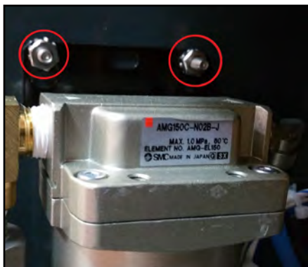
Photo 37 - Shown in red are the nuts and star washers to remove from the bracket
