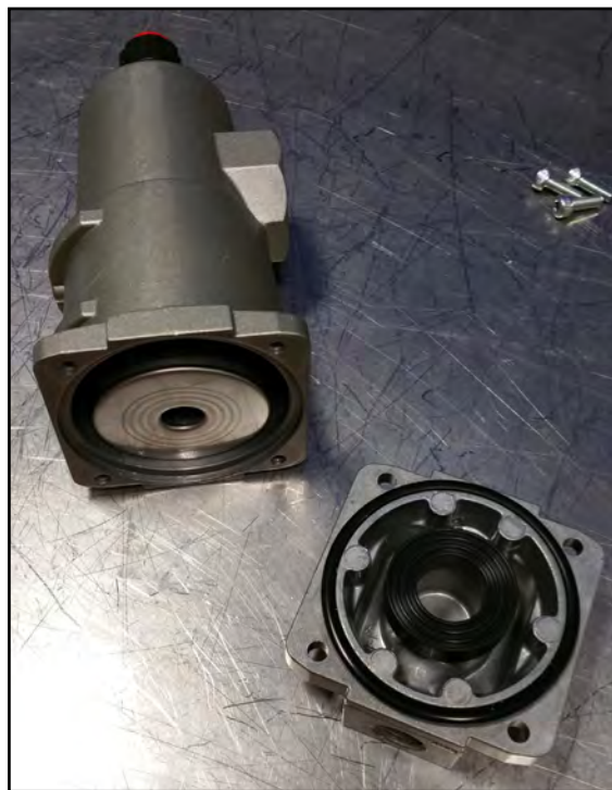
Photo 39 - Filter head removed from filter body
