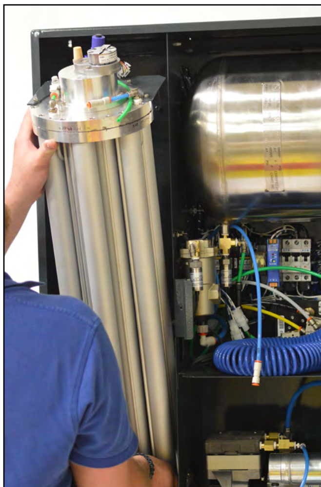
Photo 15 - Lowering the ATF unit onto the bracket.
