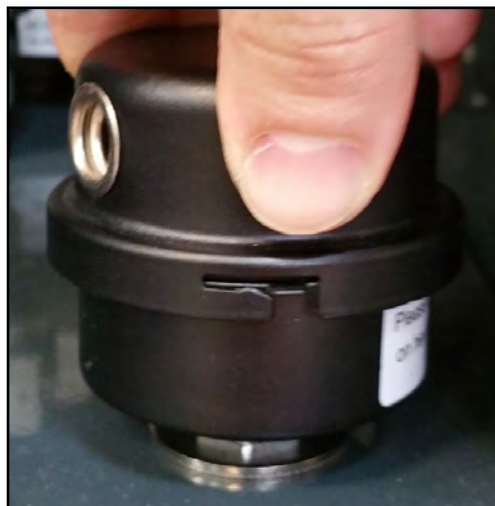
Photo 35 - Locking the filter assembly
