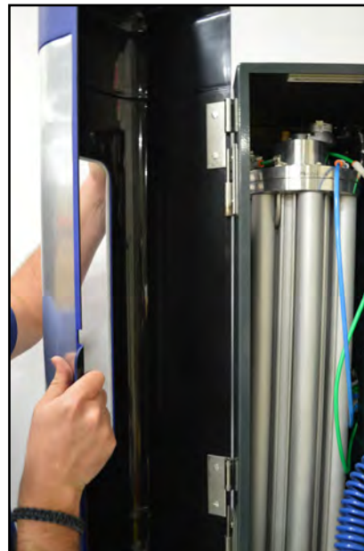
Photo 25 - Line up the receivers on the doors with the pins on the cabinet
