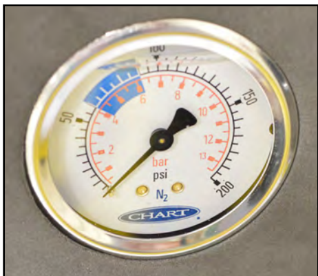
Photo 32 - Nitrogen gauge reading 0 psi
