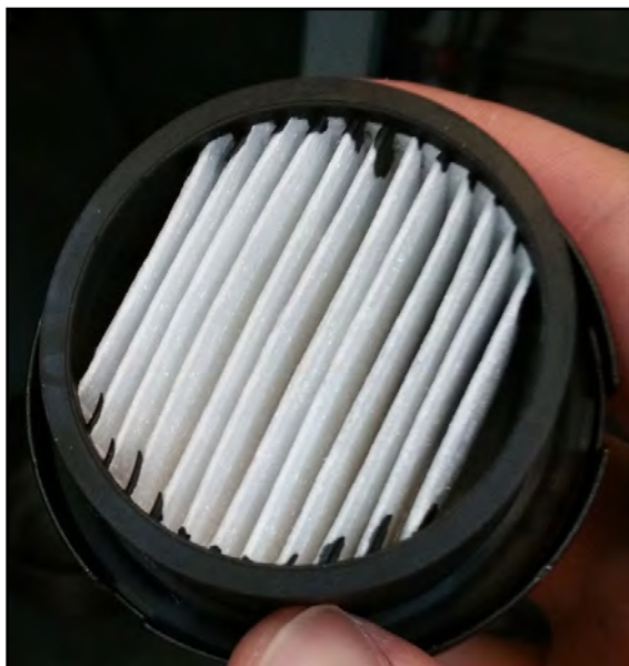
Photo 33 - Pleated filter element inside housing
