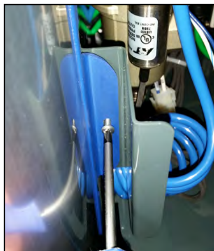
Photo 26 - Secure the left door with the small screw
