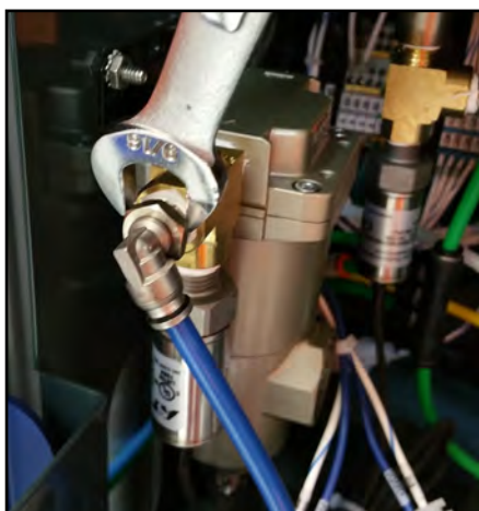
Photo 36 - Detaching push-to-connect airline connections
