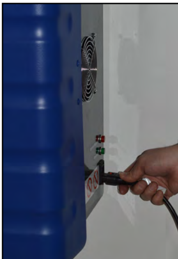
Photo 27 - Connect power cord to receptacle in cabinet
