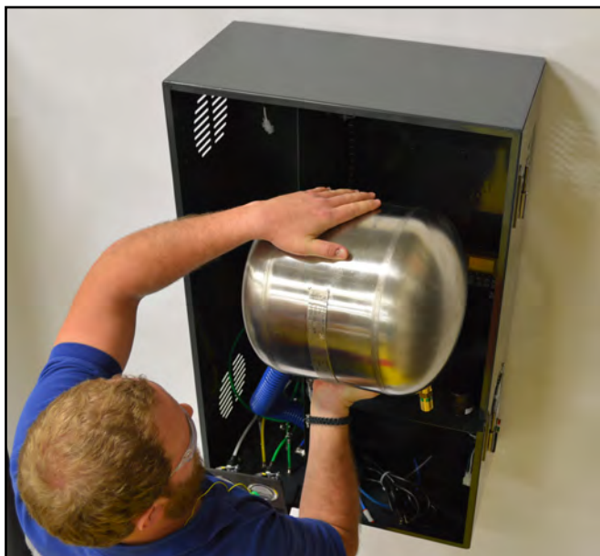
Photo 6 - Proper handling of the stainless steel N 2 tank.
