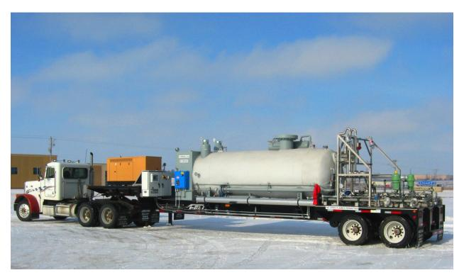
The Mobile High-Flow LNG Vaporization System (MVS-150) is designed to meet the highvolume fuel requirements of the increasing number of pressure pumps, blenders and other field equipment used in a variety of applications today.
