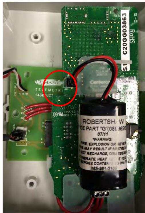
7. On the back side of the board there is a red LED that will flash. This means the system is transmitting the data.
