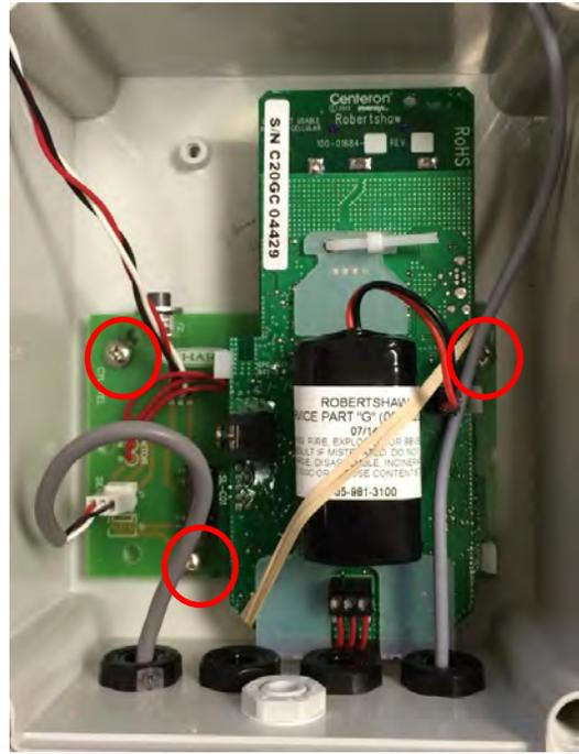
4. Plug the differential pressure sensor wire into the J1 port on the telemetry board.
