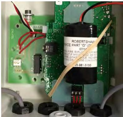
3. Secure the cellular board using the three enclosed mounting screws.
