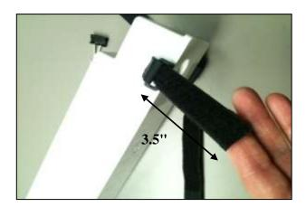
**Step 5.** Install the filter into the muffler assembly as shown by securing the bottom strap to the Velcro strip on the filter and then over top of the top strap. Ensure port on filter is not obstructed by strap.
