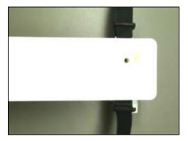
**Step 2.** Reverse the "nap" direction on the Bottom Velcro strap of the muffler assembly such that the Velcro loop material faces up.
