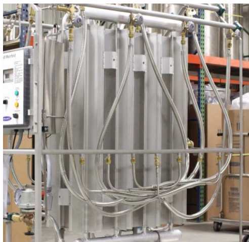
Figure 3: Hoses secured to the frame before transport
