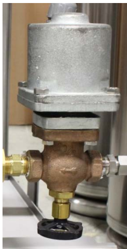
Figure 7: Solenoid with manual override
