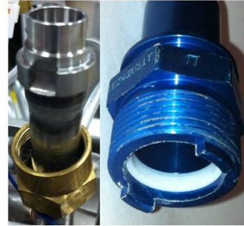
Figure 8 - - Former Posi-Lock Connection on Liberator Reservoirs
