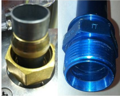
Figure 8 - - Former Posi-Lock Connection on Liberator Reservoirs
