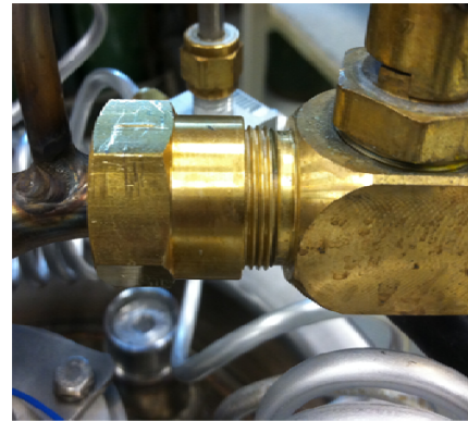
Figure 9 - - Vent Valve Connection to Manifold
