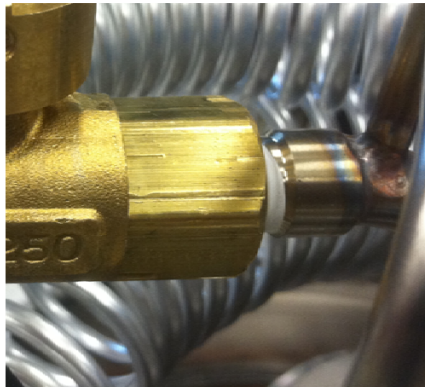
Figure 9 - - Vent Valve Connection to Manifold
