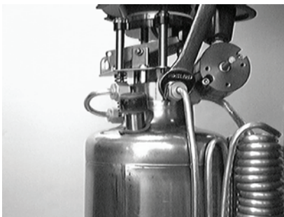
Figure 18: Warming Coil Removal
