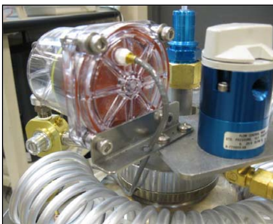
Figure 5 - - High Pressure Sensing Line Routing
