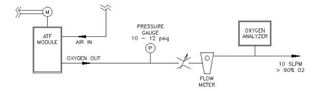
Diagnostic Test Setup for ATF Module
