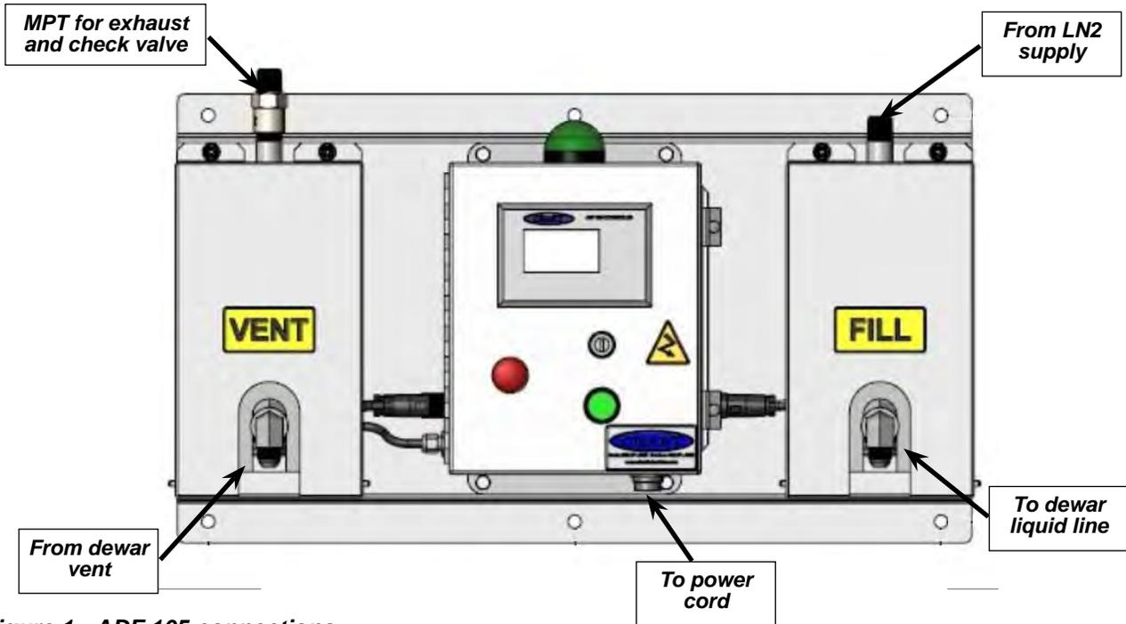
Figure 1 - ADF 105 connections
