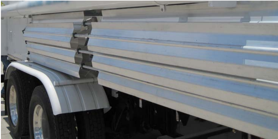
Figure 4-Orca XT-2500/2000 Pressure Building Coils
