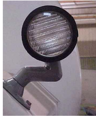
Service Lights (Exterior Cabinet Road & Curbside)
