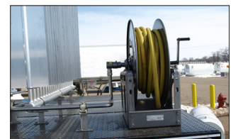
Hose Reel & 50' Gas Hose
