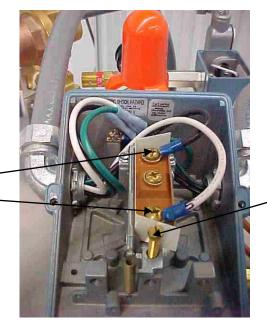
Liquid level switch adjustment
