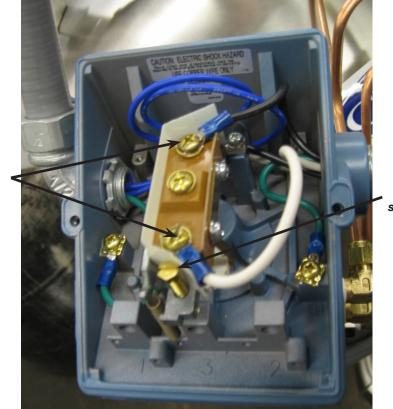
Liquid Level switch connections
