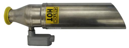
The CryoVent Exhaust Gas Heater is designed to fit on the bayonet outlet of a Chart CryoVent. The heater keeps the CryoVent outlet frost-free. The heater is designed for outdoor use in nitrogen service.
