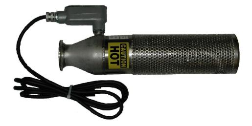
The CryoVent Exhaust Gas Heater is designed to fit on the bayonet outlet of a Chart CryoVent. The heater keeps the CryoVent outlet frost-free. The heater is designed for indoor use in nitrogen service. The nitrogen vent gas is exhausted into the room, therefore the potential for an oxygen-deprived atmosphere must be considered.
