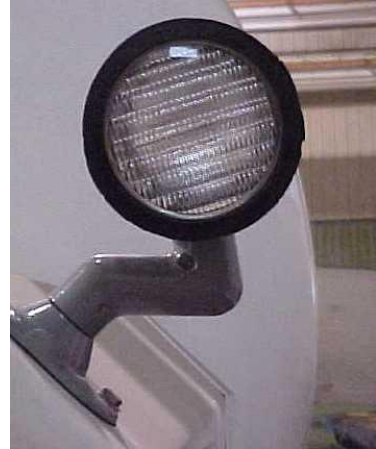
Service Lights (Exterior Cabinet Road & Curbside)
