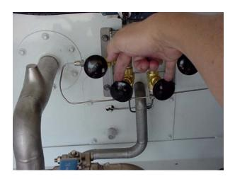
Once these lower valves are open while the outer ones are closed and the meter is switched to channel 1 the unit is now ready
