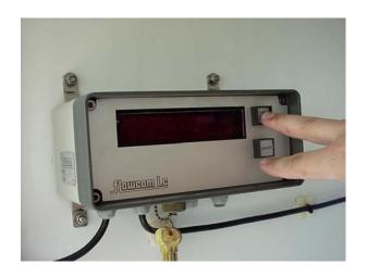
The first item flashing on the menu will be "SEL." Press the clear/print button briefly to change from channel 2 to channel 1.
