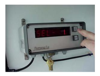
Once set to channel 1 press and hold the clear/print button until the "ex" message appears in the window. Press clear/print briefly while in the "ex" menu to exit out of the start up menu. Once 0.0 lbs appears in the window close the outer set of transmitter isolation valves and open up the inner (lower) two valves.
